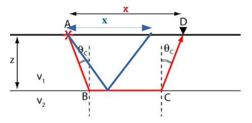
(a) Direct Wave: This relationship will be linear in x, with a slope of  $1/v_1$ . Recall that the direct wave travels along the surface at a velocity of  $v_1$ .
